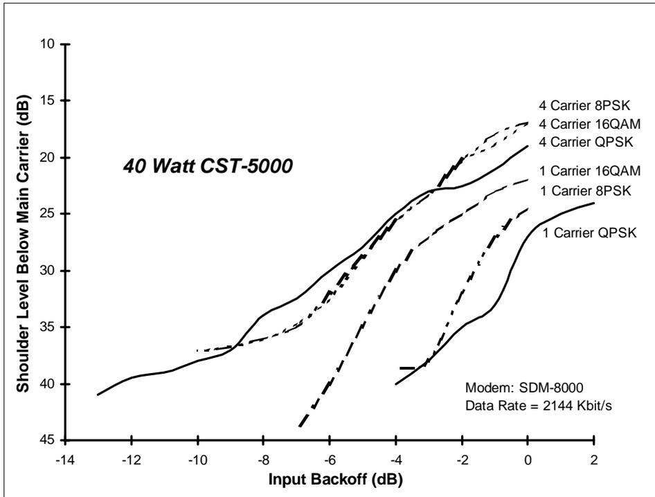
Figure 3. Shoulder Level (vs) Input Backoff
