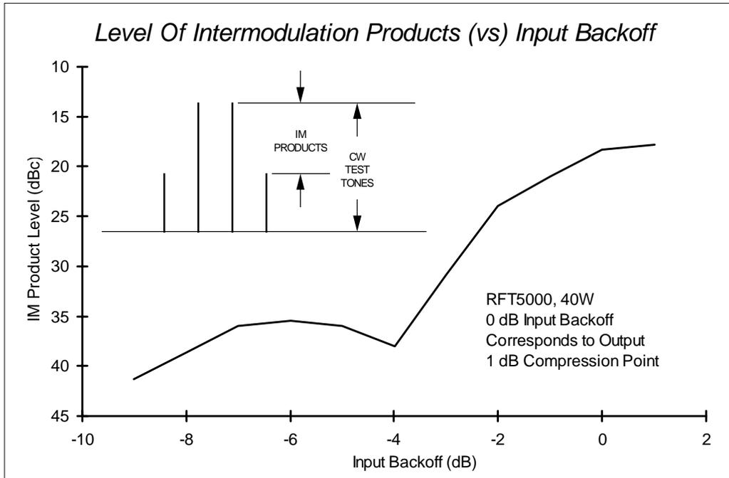
Figure 5. Intermodulation Products (vs) Input Backoff
