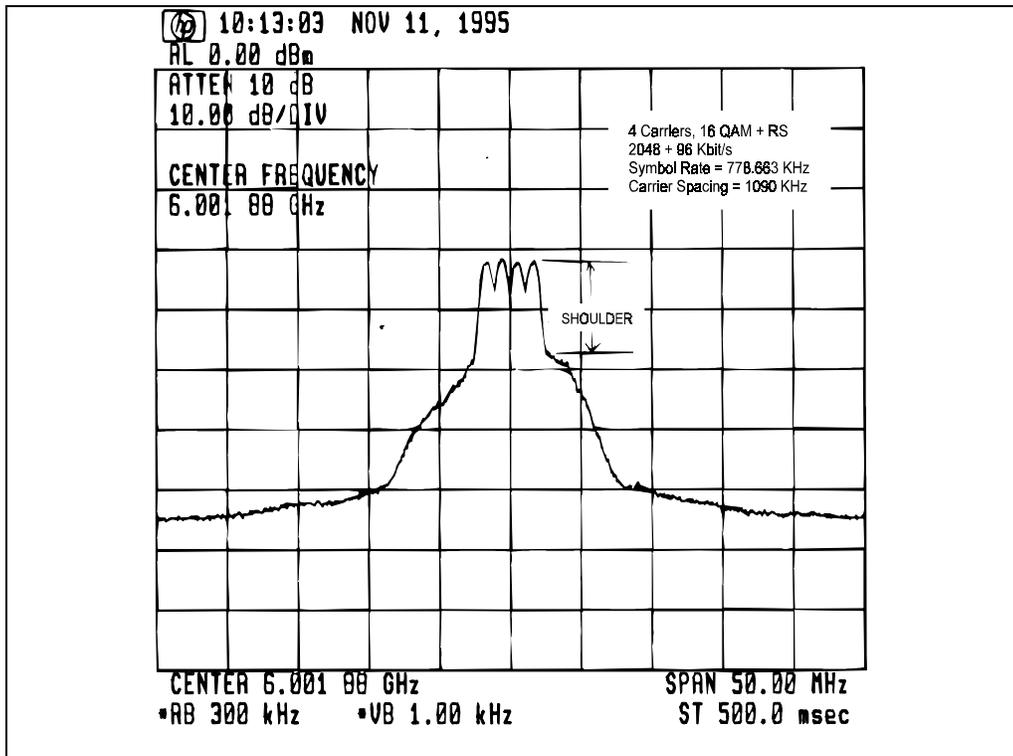
Figure 9. Four Carrier 16QAM
