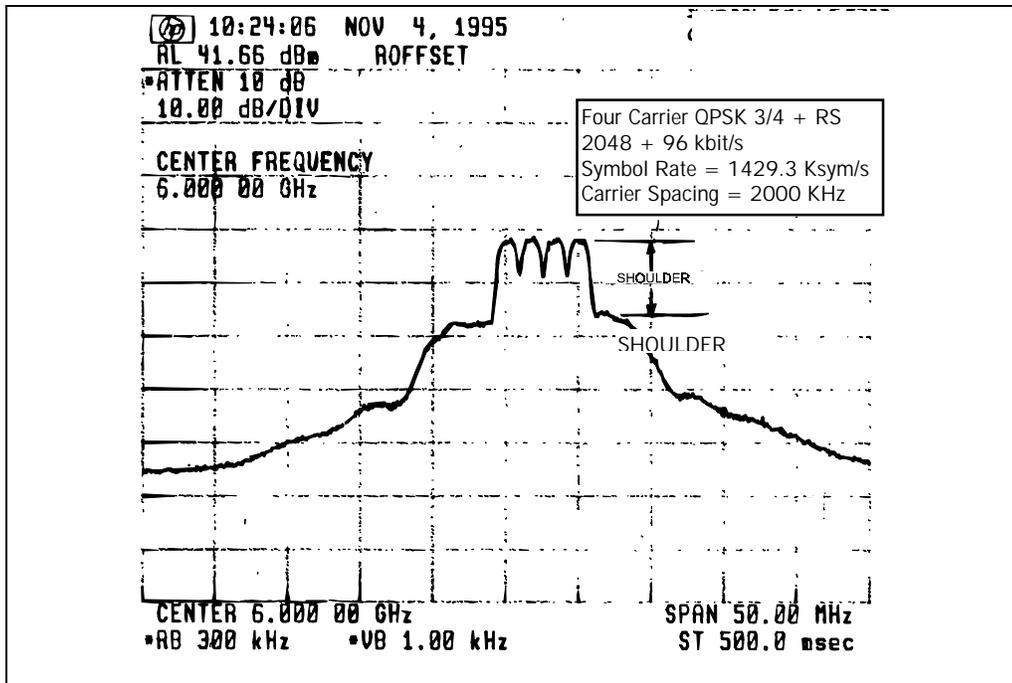
Figure 7. Four Carrier QPSK
