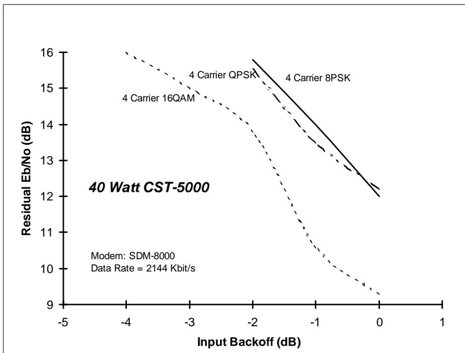
Figure 4. Residual  $E_b/N_0$  (vs) Input Backoff
